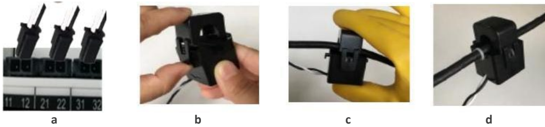
Figure 2-16 5A/2mA, 50A/40mA, 100A/40mA, 200A/40mA or 400A/40mA SCCT Installation
