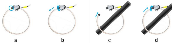
Figure 2-19 Rogowski Coil Installation Steps
